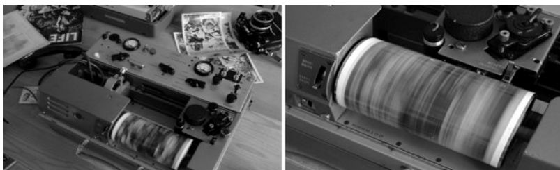
Fig. 8-7: Muirhead Picture Transmitter in operation. (Images courtesy Michael Ebert)
